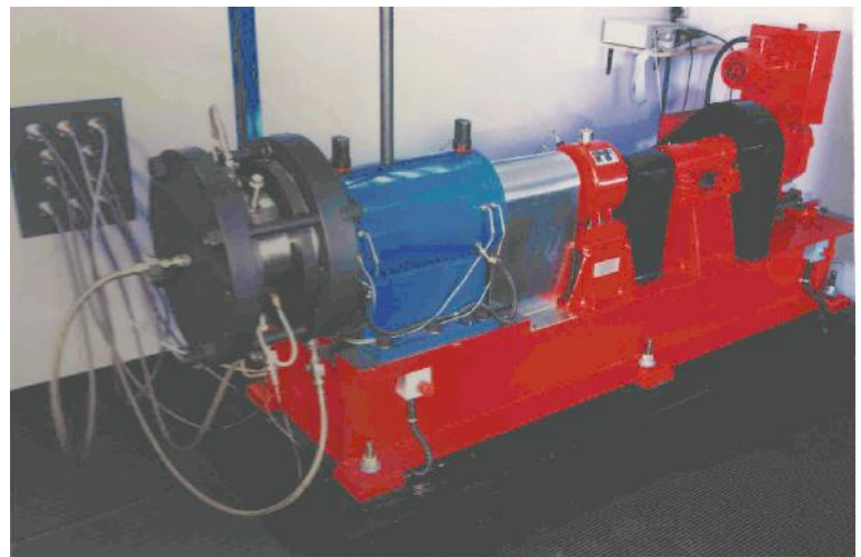
High Speed Seal Rig
