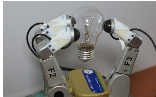
Hemispherical Sensors mounted to Robot hand
