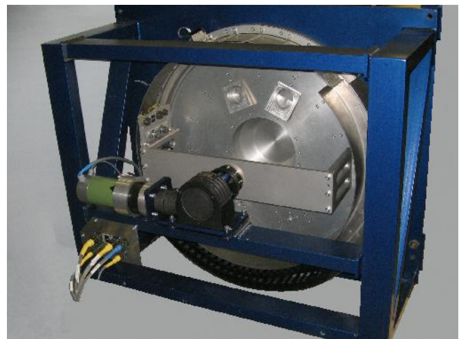
Circumferential Traverse System Mounting Hub and Support Framework
